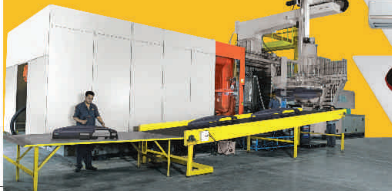
3200T Machine with robotic pick-up and online finishing & assembly for moulding large components.
